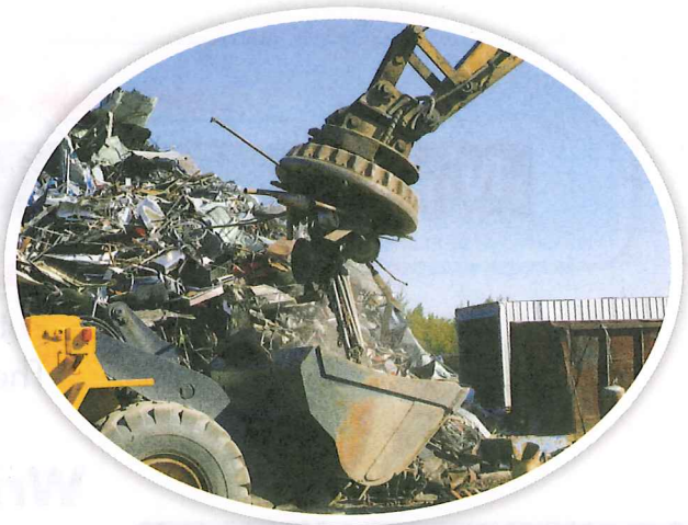
An electromagnet separates metal from other materials.
