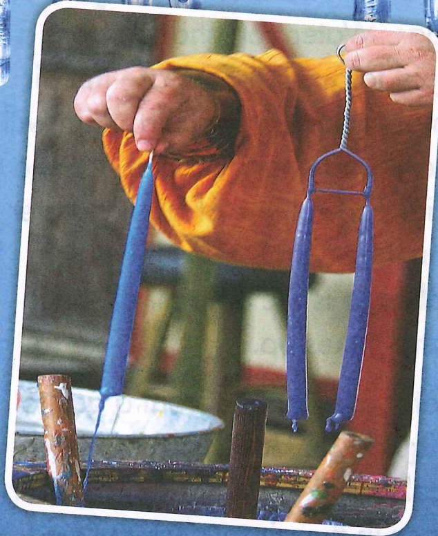
Some candle makers dip strings in and out of melted wax to make candles.
